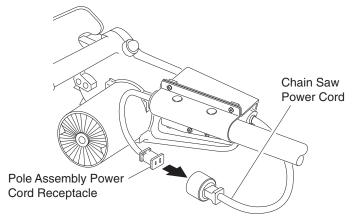
Figure 3 - Connecting Chain Saw Power Cord to Pole Assembly Power Cord
